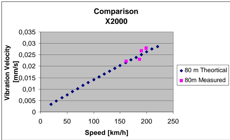
To check for the prediction formula, the error mean  $\bar{\Delta}$  will be calculated and the standard deviation  $s_{\Delta}$  as well, for the X2000 trains.
