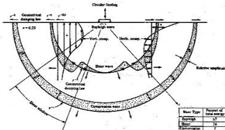
Figure 3.1 Wave propagation in the ground [29].
