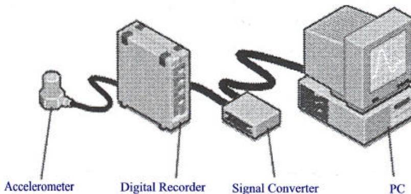
**Figure 7.1** Connection to convert the analog signal to digital signal
