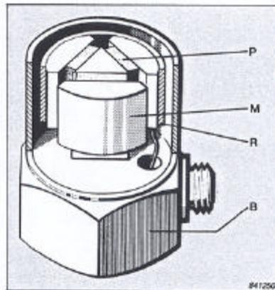
**Figure 6.6** Piezoelectric accelerometer, (*the unique Brul & Kaer, Delta shear design*).
