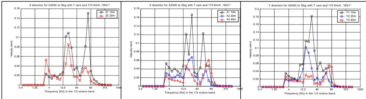
Figure 7.11 Measurements results for X2000 train, to show the dominating direction.
