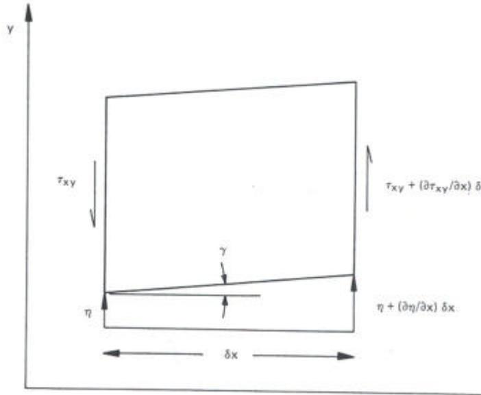
**Figure 3.6** Displacement; shear strain, and transverse shear stress in pure transverse deformation.
