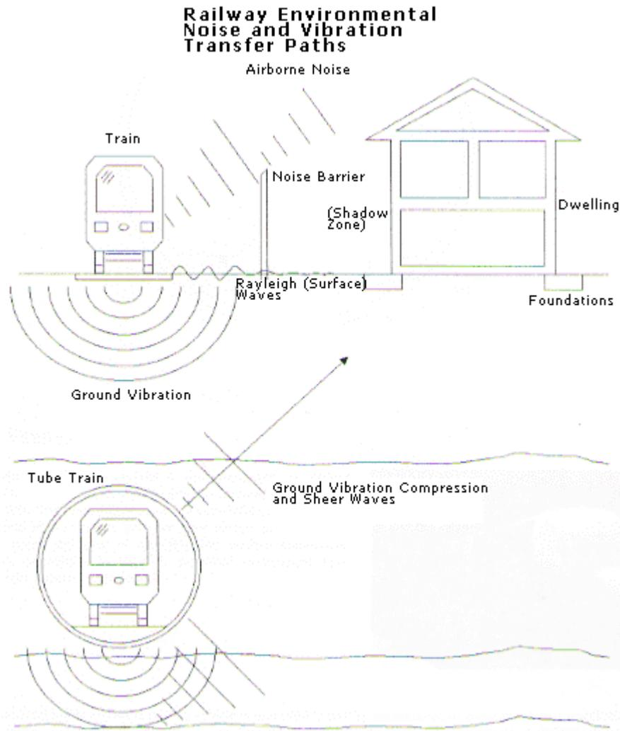
**Figure 0.1** Vibration generates by the railway and propagates to the urban area.
