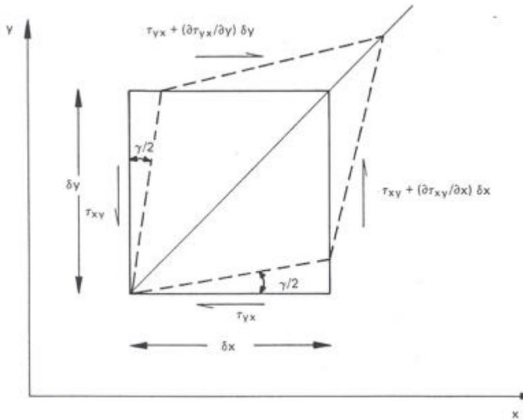
**Figure 3.5** Pure shear strain and associated shear stresses.
