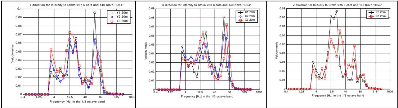
Figure 7.9 Measurements results for intercity train, at the same site and position.
