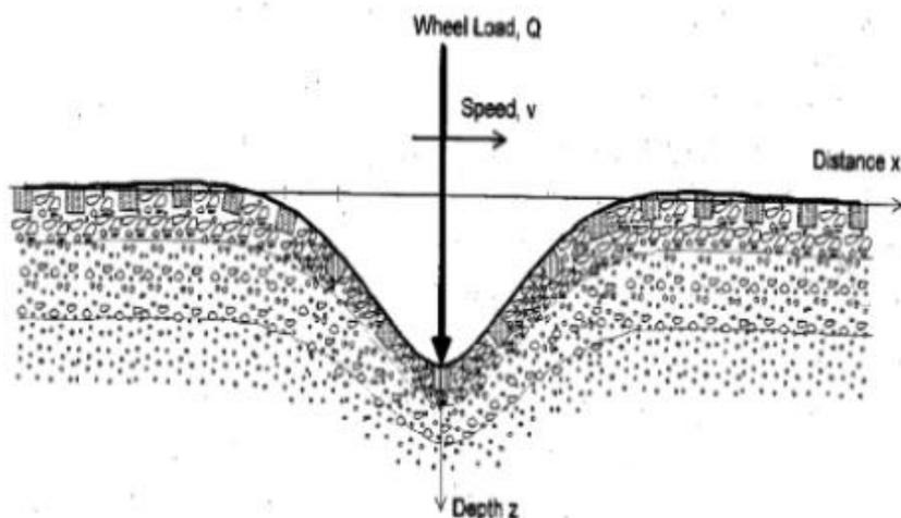
**Figure 1.1** The wave pattern moving with the train direction. [29]
