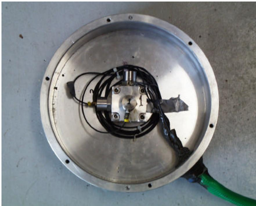
**Figure 6.5** Three directional accelerometer mounted inside waterproof box.
