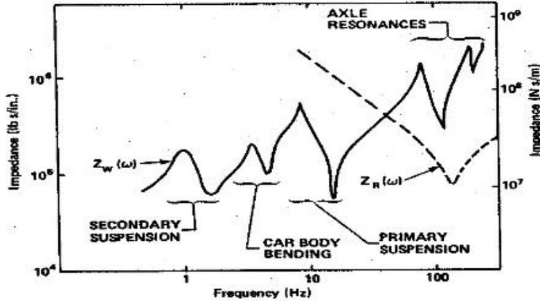
**Figure 1.3**  $Z_w$  and  $Z_R$  for a typical transit car operating on typical tie and ballast rail.
