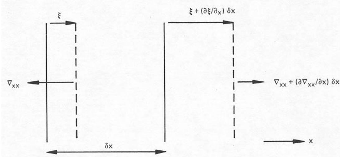
**Figure 3.3** Displacement from equilibrium and stresses in a pure longitudinal wave.
