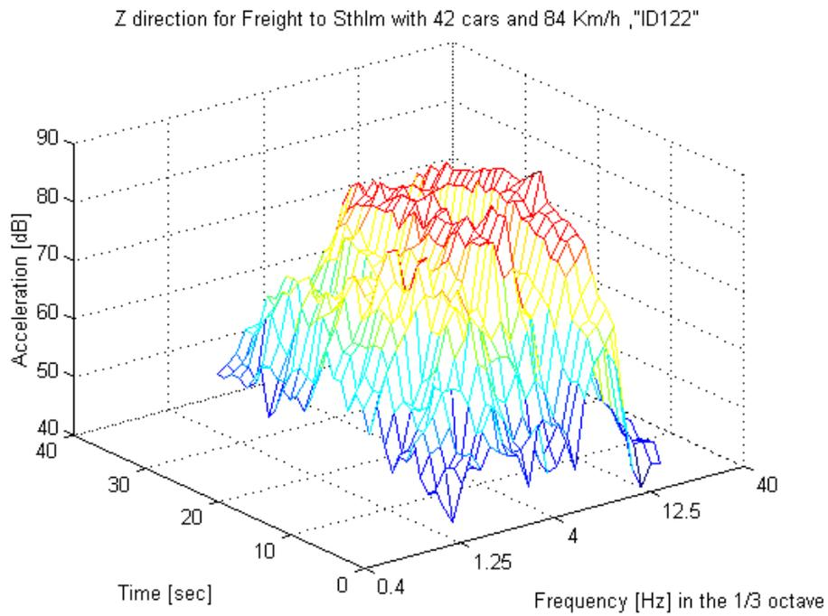
**Figure 7.7** Acceleration levels [dB] against 1/3 Oct. band frequency. The results for the same Train in Fig.7.6
